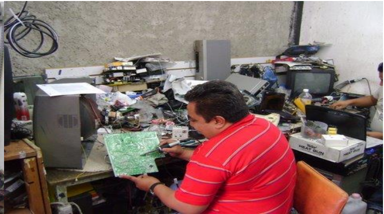
Soldering an integrated circuit board to a PCB in a TV repair shop in downtown Mexico City, Mexico Source: Kahhat, R. 2010
